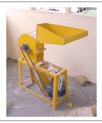
Small HAMMERMILL with interchangeable sieves.
