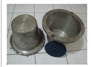
A two piece aluminum **MOLD** is the only specialized component of the press.
