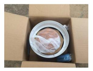
9. The receptacle lid is placed in a plastic bag and placed inside the second receptacle piece, on top of the filter.
