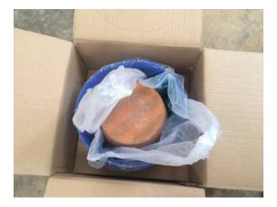
7. A second cardboard form is then placed over the filter pot and inside the receptacle.
